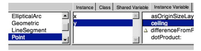
When you do this the third list pane from the left contains a list of the instance variables of the class, in this case x & y. When you select one of the variables the fourth pane lists all the methods in the current class that access that variable.
